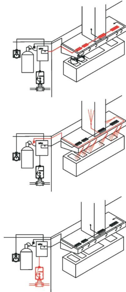
The combination of the Amerex KP system and an Amerex Model B260 or B262 Wet Chemical extinguisher provides restaurants with a “ONE-TWO” attack against the threat of business loss due to cooking operation fires.
